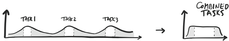
Figure 7.6: Illustration of the energy pattern Batch Operation. Energy usage can be reduced by combining the execution of different tasks.
